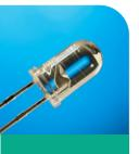
LEDs have changed the way of lighting streets, homes and workplaces in the 21st century. LEDs are highly energy efficient, as they convert electricity directly into light. Polycarbonate is used for the housing and internal parts of LEDs. Its outstanding transparency, in combination with it's break resistance, high heat resistance, and inherent non-flammability, allows for LEDs characteristic brightness in spreading the light and for their energy efficiency.
